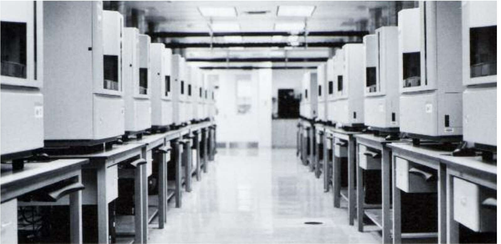
DNA SEQUENCER LABORATORY SEPARATES AND DETECTS FLUORESCENT LABELED DNA SEGMENTS
