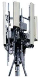
5G Base Station
