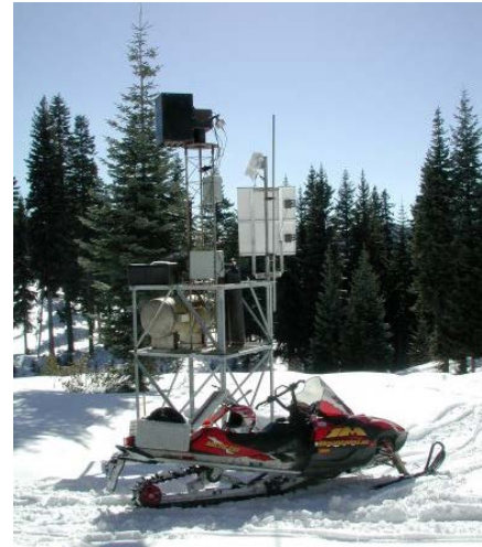
Cloud seeding ground generator.
