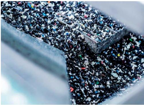
Shredded PP waste, here shown as chips (shown above) are converted into an rPP compound (shown right). Such rPP compounds are used directly by automotive suppliers and converted into car parts.
