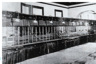
Magnetic parallel multiple telephone switchboard
