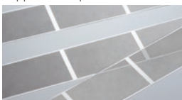
Metal masks for OLED
