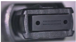
Connector terminal (ferrule) cross-section
