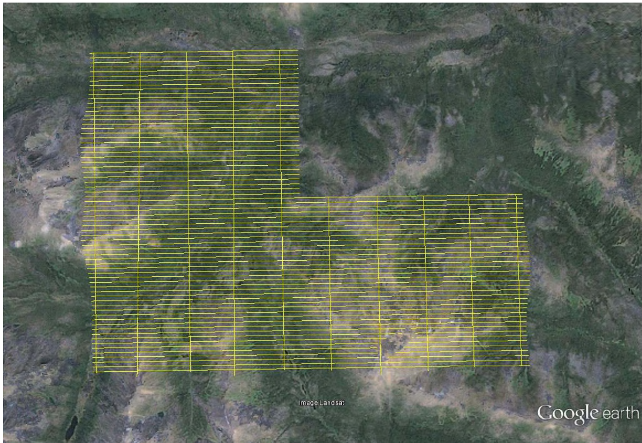
Figure 16: Flight lines overlain on a Google Earth Image (Geotech Ltd. 2014)
