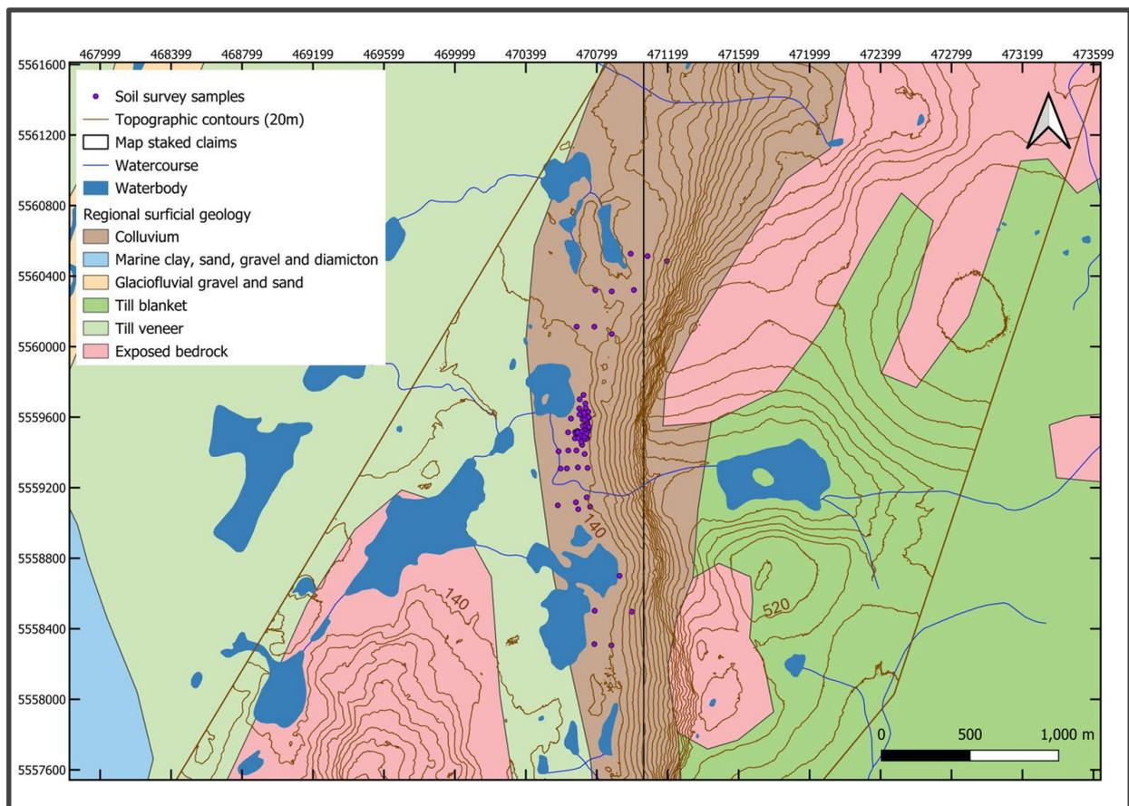
**Figure 5 Newfoundland government surface geological map with the location of the maiden soil samples and topographic contours. NB: The dense cluster of sample points is the Talus high-grade uranium soil anomaly.**
