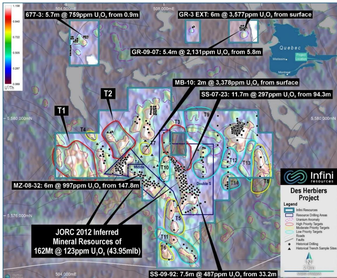
**Figure 8 The Des Herbiere Uranium Project in plan view depicting anomalous radiometrics (U<sup>2</sup>/Th), historical drilling and trench channel sampling. Note the several large target areas that have never been drill tested.**
