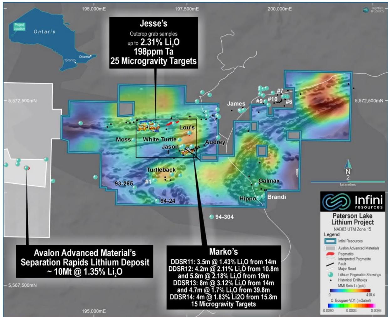
**Figure 11 Location of the Paterson Lake Lithium Project depicting the microgravity survey locations overlain with 1VD drone magnetics, MMI soil sampling, mineralised outcropping pegmatites and historical drillhole mineralisation. The Avalon Advanced Materials/Sibelco JV lithium deposit of ~10Mt @ 1.35% Li<sub>2</sub>O lies within 2km of the claim boundaries<sup>1</sup>.**
