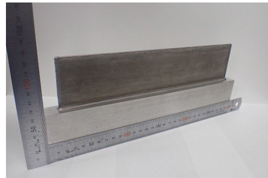
Sample of magnesium alloy for additive manufacturing
