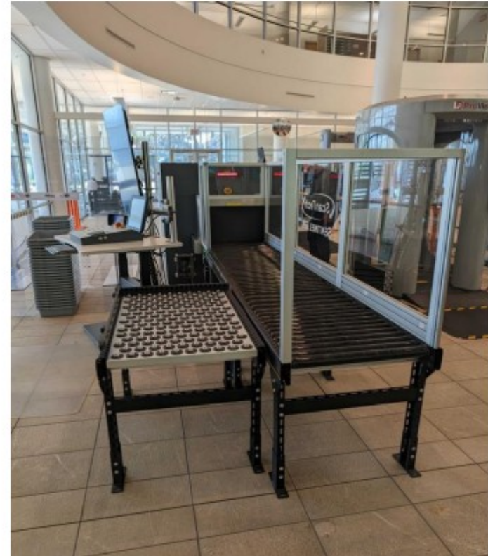
SENTINEL CT Scanner at Darlington Nuclear Power Plant
