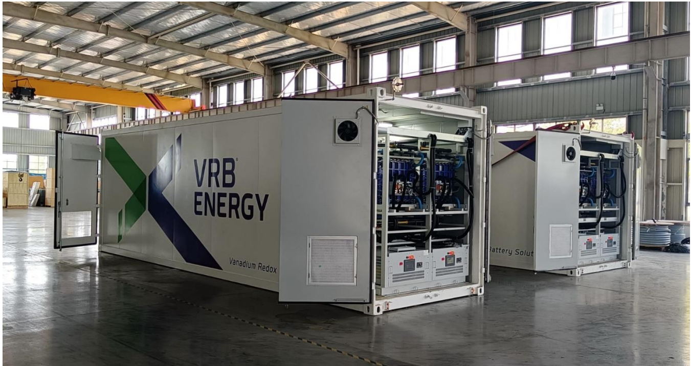
Photo 1: VRB Energy’s Pod 100 VRB-ESS® vanadium redox flow battery in production.
