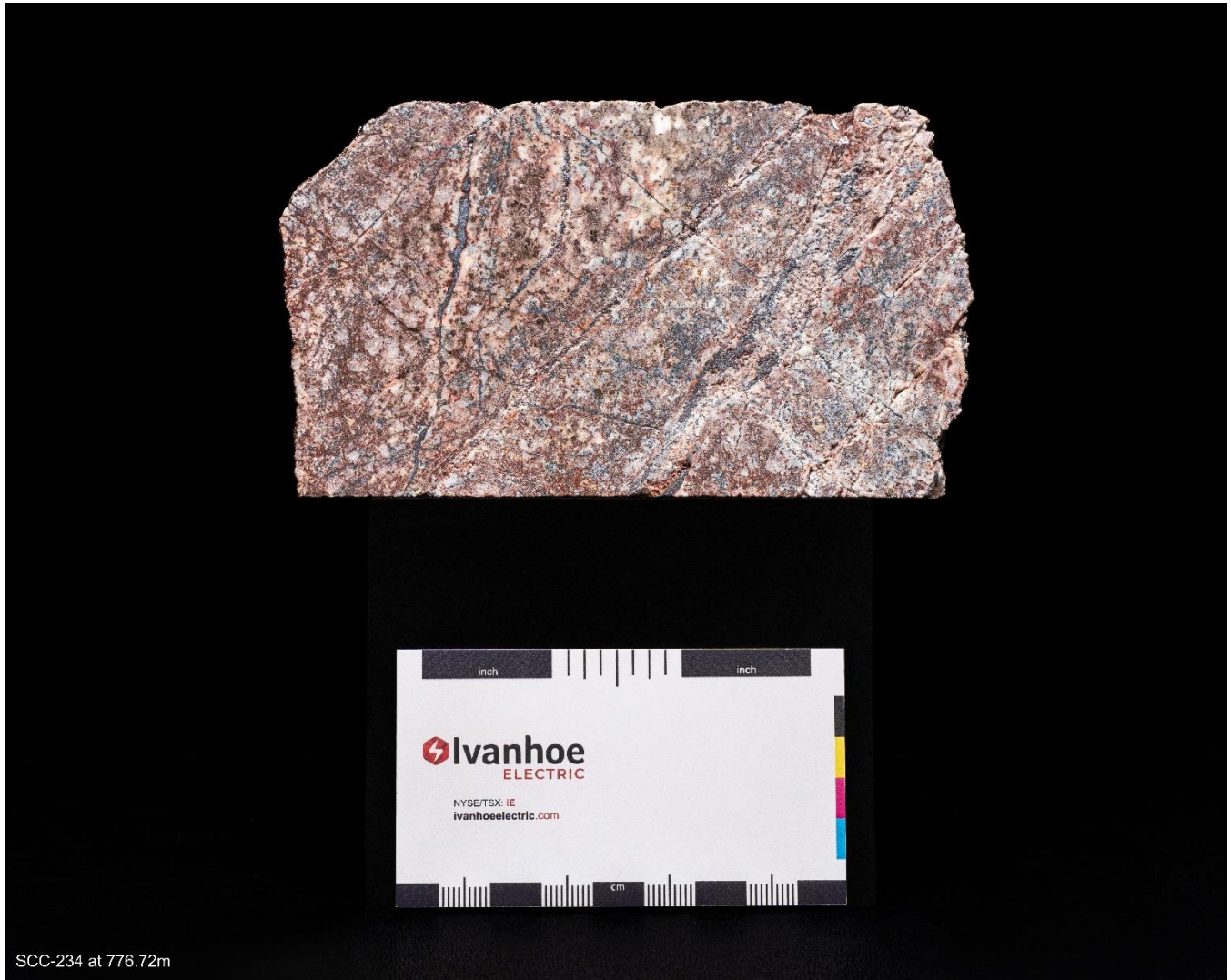
Photo 1. Drill core from infill drill hole SCC-234 at 776.72 meters showing intense steely-gray chalcocite (a floatable mineral that is approximately 80% copper by weight) enrichment mineralization in veins and disseminations.
