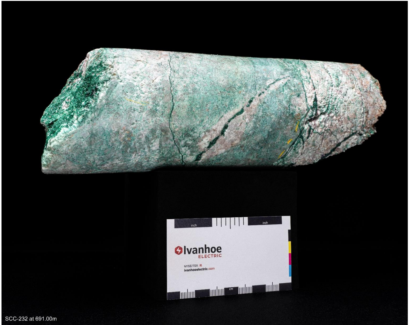
Photo 2. Drill core from infill drill hole SCC-232 at 691.00 meters showing intense dark green atacamite (a leachable mineral that is approximately 60% copper by weight) mineralization.
