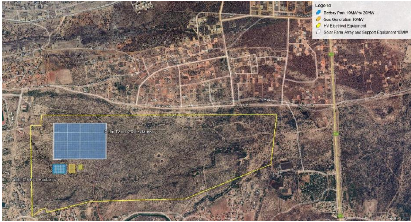
Figure 5 - Schematic of solar and gas hybrid plant layout on Serowe site
