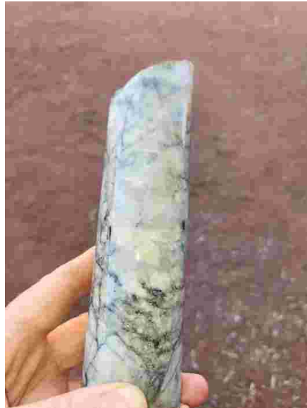
Figure 2: MPDD003 Drill core, from 68.8 m, MPL21-656 (0.02% Li 2 O), a Monzogranite made up of roughly 30:30:30 Plagioclase : Quartz : Microcline, the remaining 10% being Muscovite. The yellow/greenish minerals in the sample appear to be saussurite, a potential hydrothermal alteration product.
