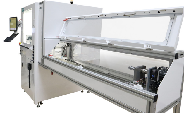
MediCoat system for coating drug eluting balloon catheters with anti-restenosis drug polymer solutions.
