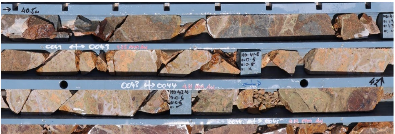
Figure 4. Brecciated volcaniclastic with colloform quartz infill associated with gold mineralisation in PCDD001 (interval 40.5 m to 43 m)
