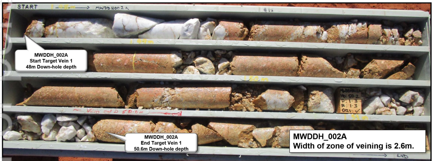
Figure 5. Main quartz vein intercept in diamond drill hole MWDDH_002A at approximately 50m down-hole depth.
