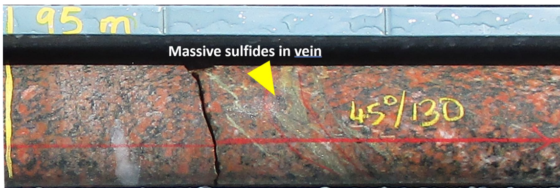
Figure 1. New zone identified below target vein containing quartz veining and massive sulphide veining. The vein above is an example of a pyrite-rich massive sulphide vein in MWDDH_002A.
