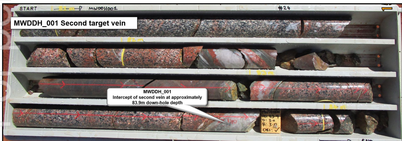
Figure 7. Second vein intercepted in MWDDH_001. Three small quartz veins are evident in the section of core shown here but the small vein at 83.9m depth shows characteristics similar to the second intercepts in the adjacent drill holes. Note that the angle of intercept is not perpendicular to the drill hole, therefore the true width is not equivalent to the intercept width.
