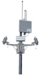
Drone Detection Radar External radar detection system provides estimated position of the intruder drone
