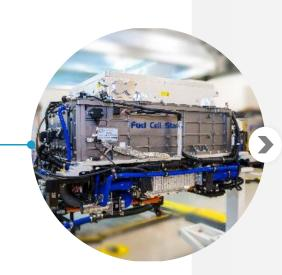
Hyzon's single stack 200 kW FCS shows significant benefits vs. traditional approach of two ~100 kW fuel cells
