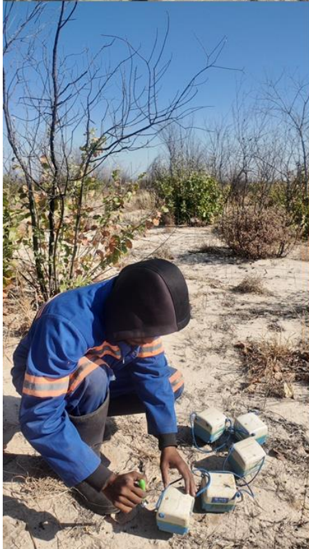
Figure 1. (Top) 1.5t accelerated weight drop source; (lower left) Smart Solo passive seismic node layout; (lower right) Stryde™ active seismic node deployment.
