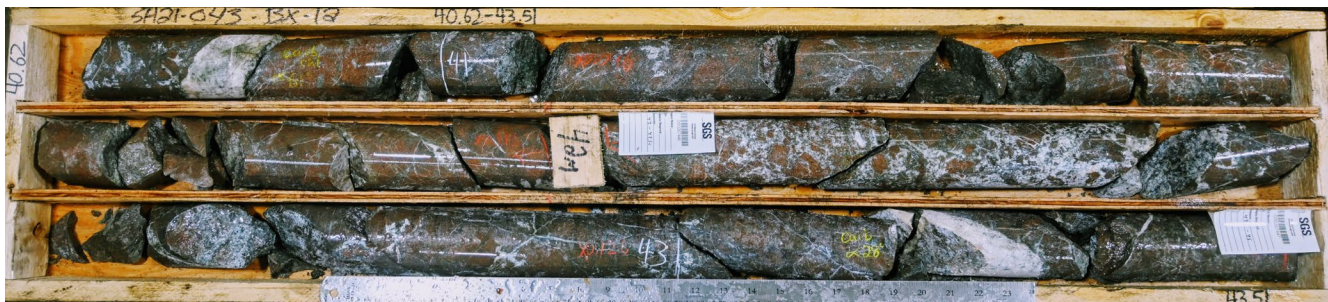
Photo 1. Mineralization Encountered in Drillhole SH21-043 from 40.6 – 43.5 m; Sample from 42.0 – 43.5 m (1.5 m) Grading 9.84 g/t Au and 443 g/t Ag [15.38 g/t AuEq*] .
