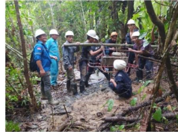
Shot hole drilling
