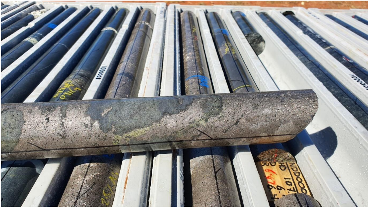
Figure 3. Semi massive sulphide from approximately 106m downhole in NDD0008, showing the interaction of the sulphides with countryrock xenoliths, and clots of remobilised chalcopyrite.
