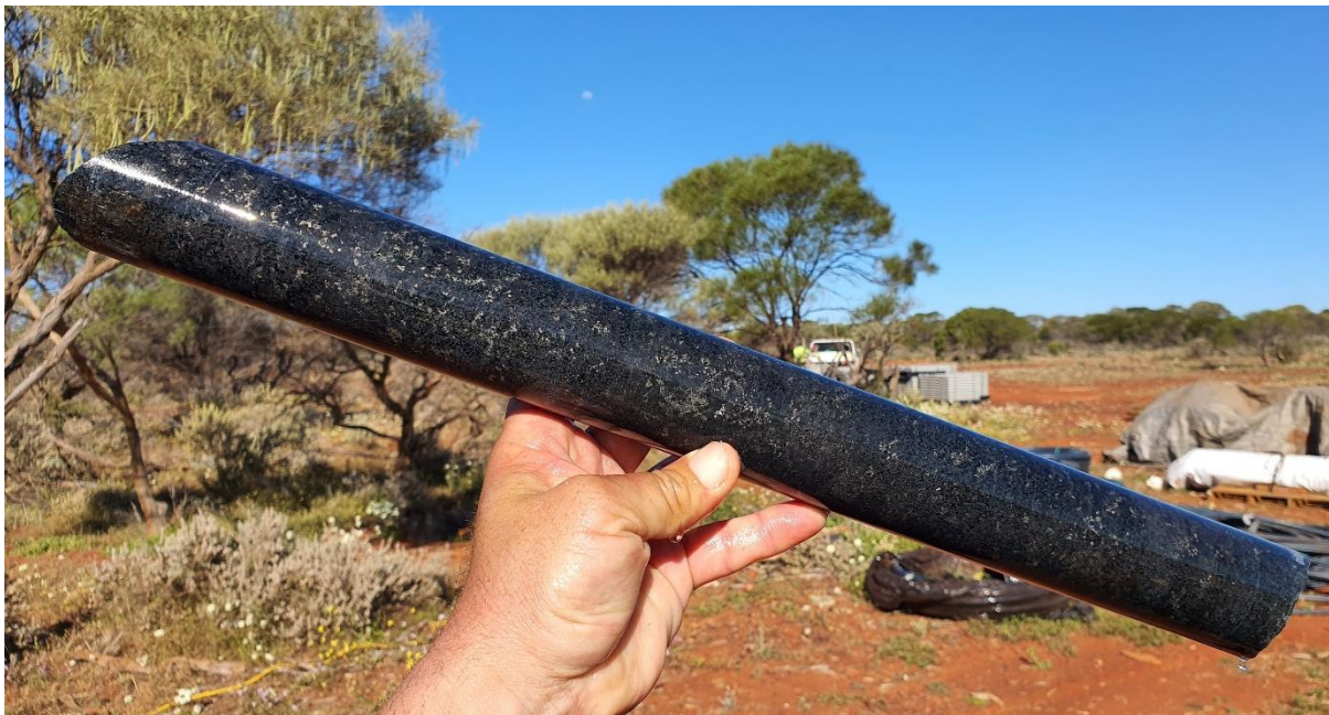
Figure 1 Cumulate textured high MgO ultramafic with disseminated and blebby magmatic sulphides in NDD0008 from approximately 89m downhole.
