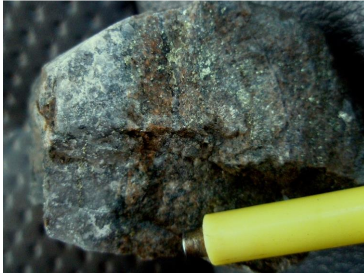
Figure 2 PEED001 at 128m - Sheeted Quartz-Chalcopyrite-Magnetite Veins
