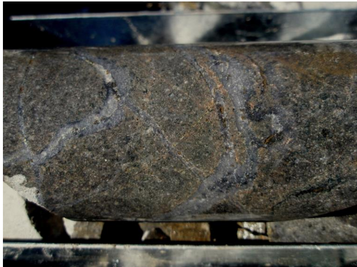
Figure 3 PEED001 at 142m - Quartz Stockworking
