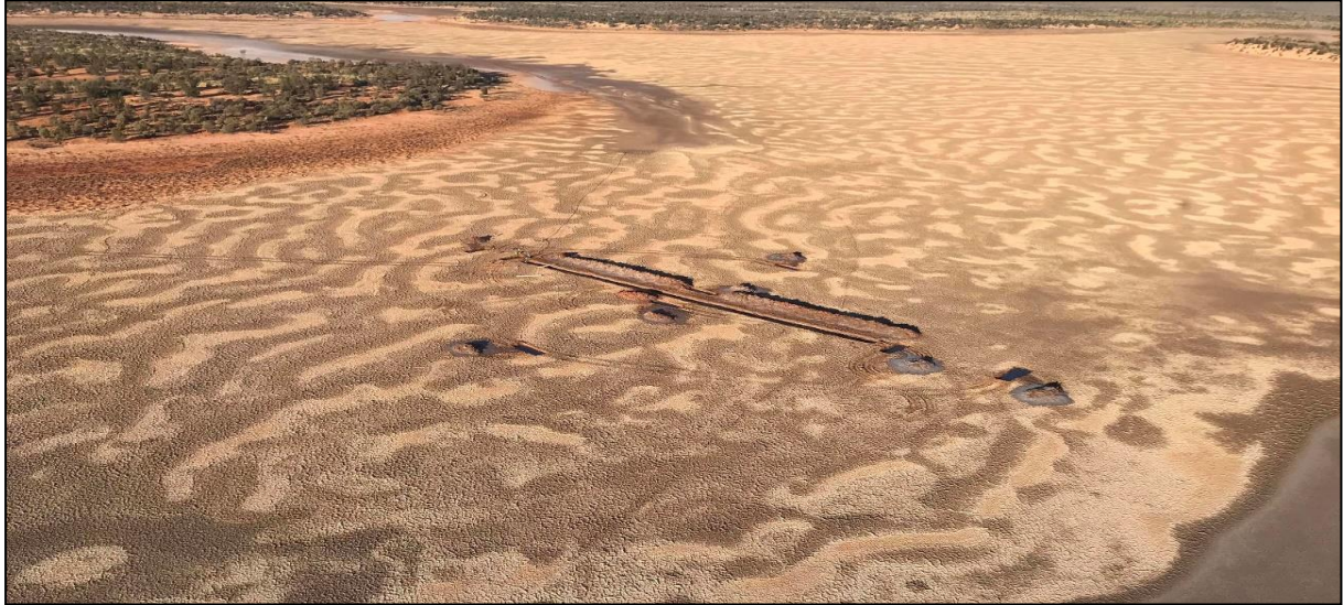
Figure 2: Trial Trench one with surrounding monitoring pits
