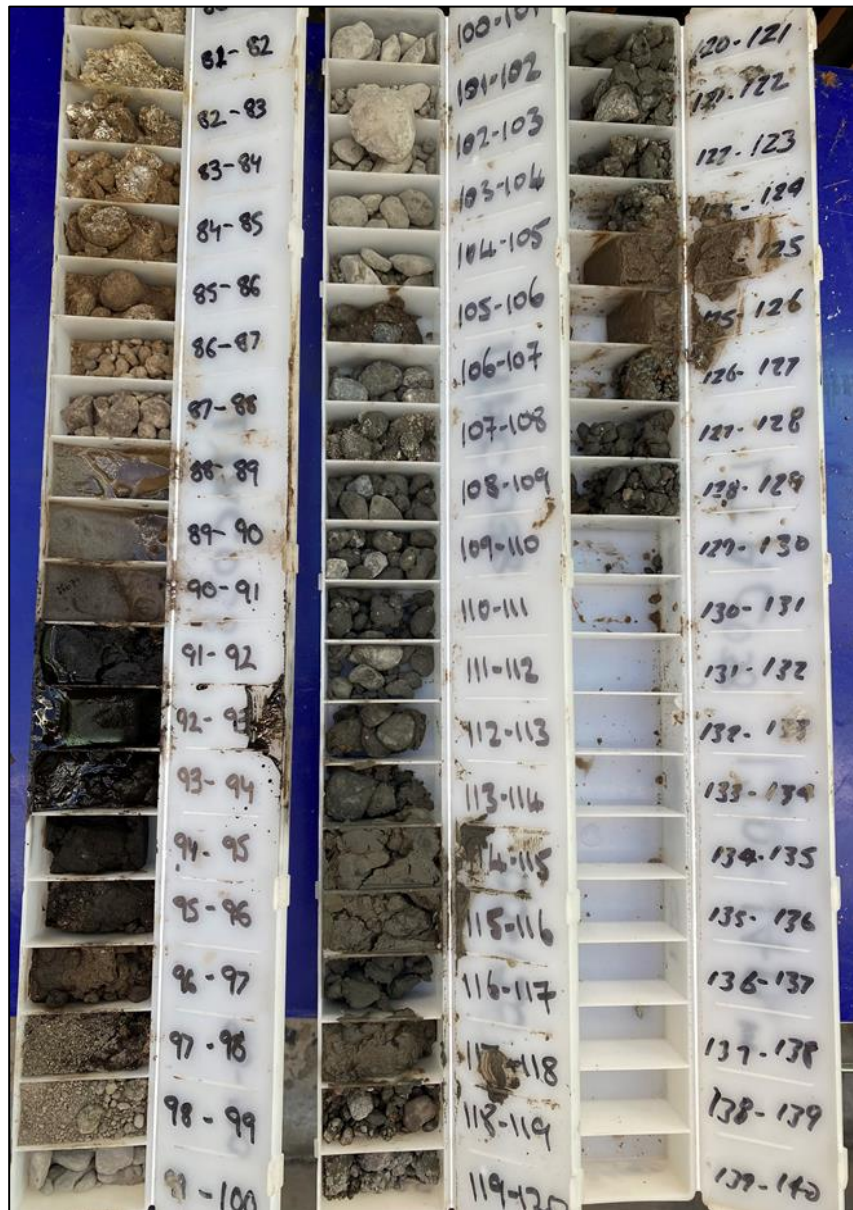
Figure 8: Chip trays showing the basal aquifer sequence (86 to 129m - gravel, fine sand, silt and minor clay)
