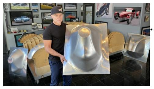
Custom classic car influencer Rob Ida of Rob Ida Concepts in New Jersey is using Desktop Metal's Digital Sheet Forming (DSF) technology on the Figur G15 Pro to create components for a 1955 Tucker Carioca, a vehicle concept from legendary carmaker Preston Tucker that never made it from drawing to production. Details of the project are featured in a new video available at TeamDM.com/TuckerCarioca (Photo: Business Wire)
