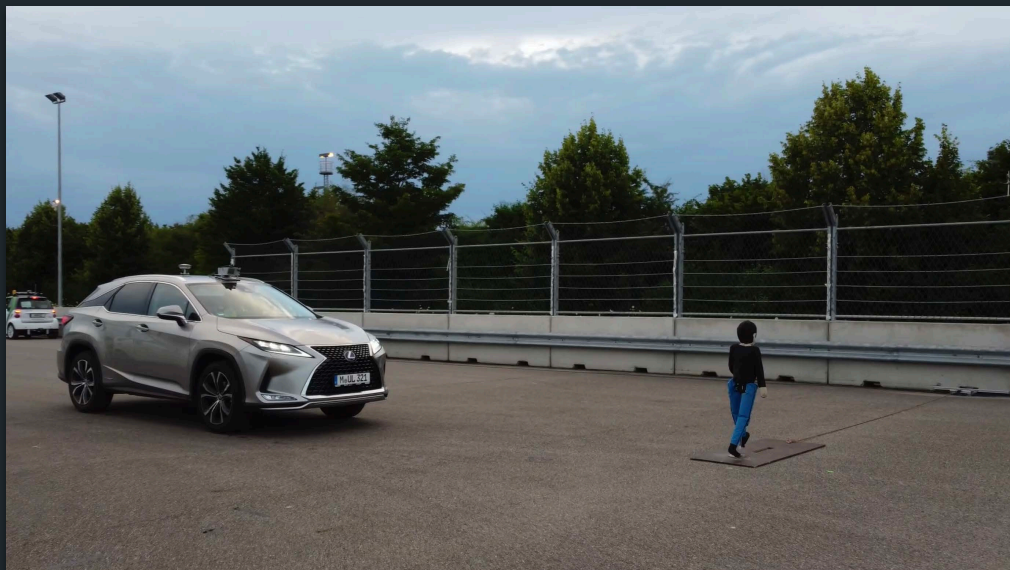
Luminar test vehicle preventing a collision in an NCAP scenario of a moving pedestrian
