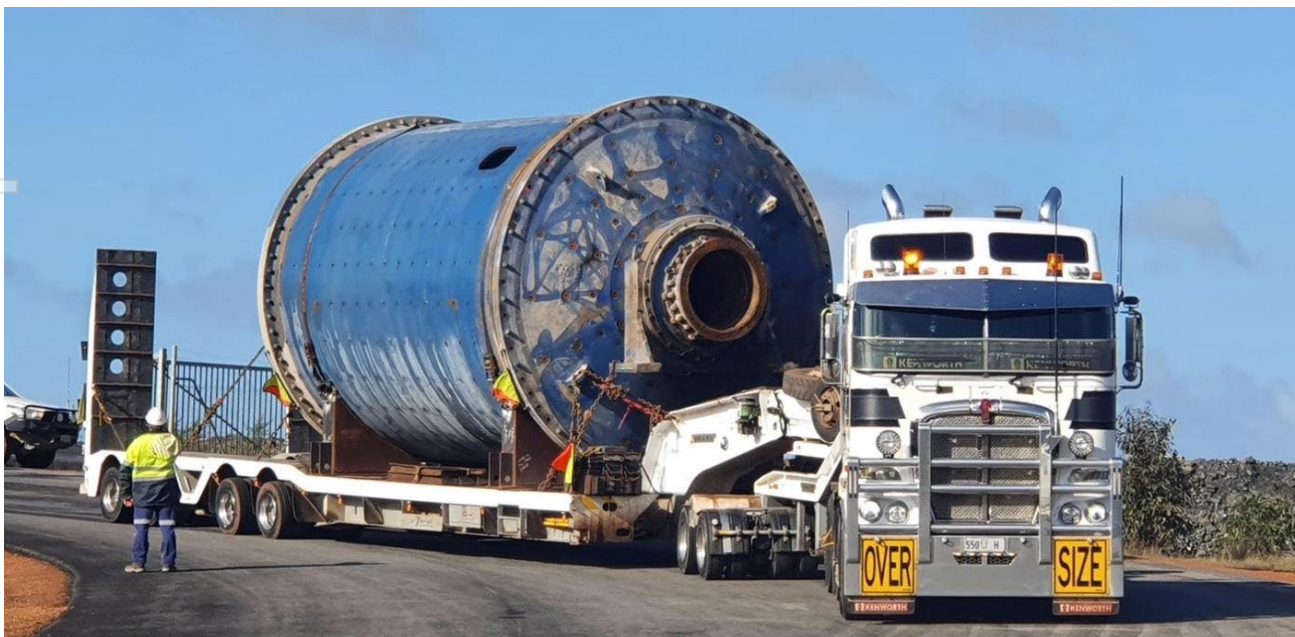
Figure 7: 1.85MW Outokumpu ball mill on the road to Kalgoorlie
