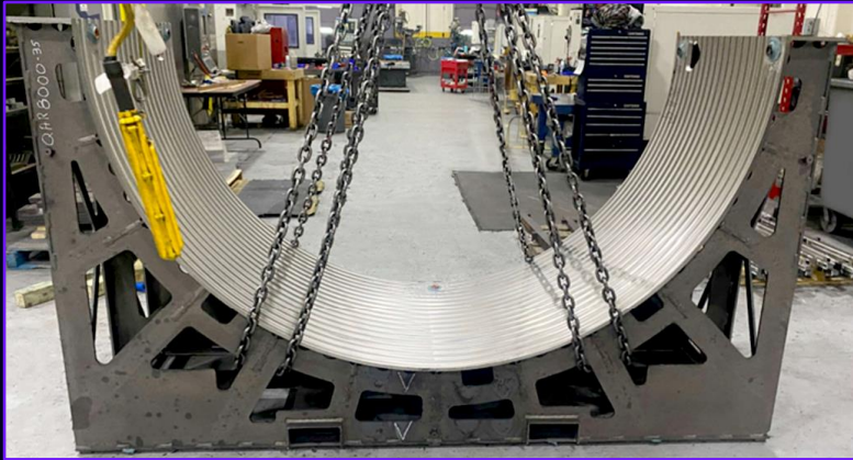
Main Oxidizer Tank lower panel
