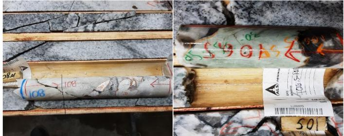
Figure 3: Spodumene crystals evident in CAD56 drill core at 106.5m and 108m, Dyke B
