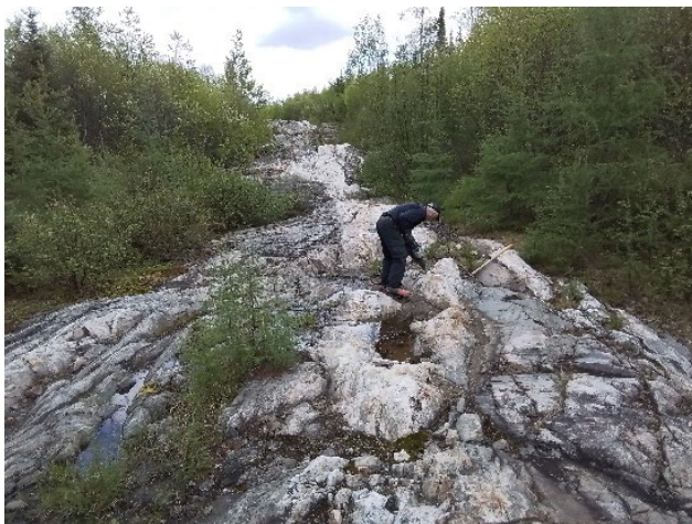
Figure 7 Papitose prospect, Dyke 1 stockwork quartz veining with disseminated chalcopyrite (local aggregations to 5%)**
