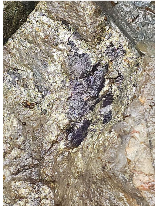
Figure 6 Chalcopyrite-pyrite-pyrrhotite-covellite(?) massive sulphide vein at the Chevrier Prospect. Photo width 50cm. Estimated 70% sulphides within vein**.
