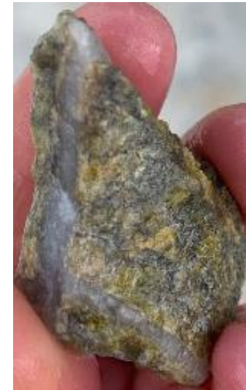
Toora West aircore chips – quartz veins with K-spar selvages
