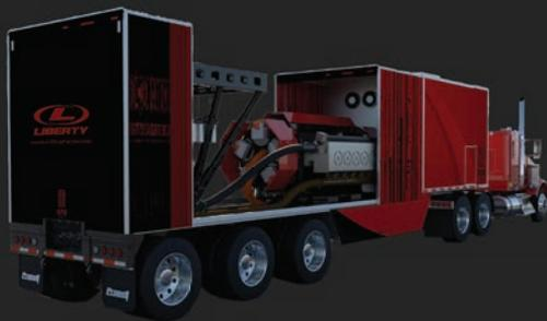
digiFrac is our fully electric frac system, featuring the industry's lowest fuel consumption and emissions per HHP-hr. Designed to allow flexibility depending on available power sources at each location, it can run on electricity generation from the grid, on-site natural gas-powered generators, or any combination of the two.
