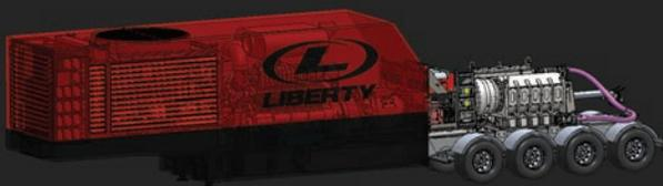
digiPrime is the world's first natural gas hybrid high-pressure frac pump utilizing reciprocating natural gas-fueled engines. Powered by a Rolls Royce engine with 45% thermal efficiency, there is less mechanical efficiency loss than a conventional electric fleet, and 29% less fuel consumption than competing technologies.
