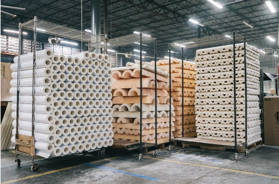
Top: TruTeam insulation installation at residential location. Bottom: Mechanical insulation inventory at fabrication facility
