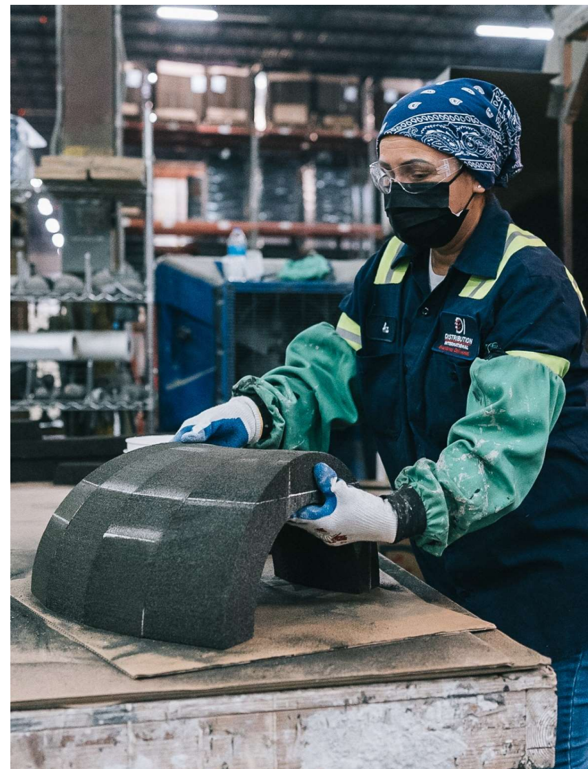
Custom fabrication of mechanical insulation at Distribution International.
