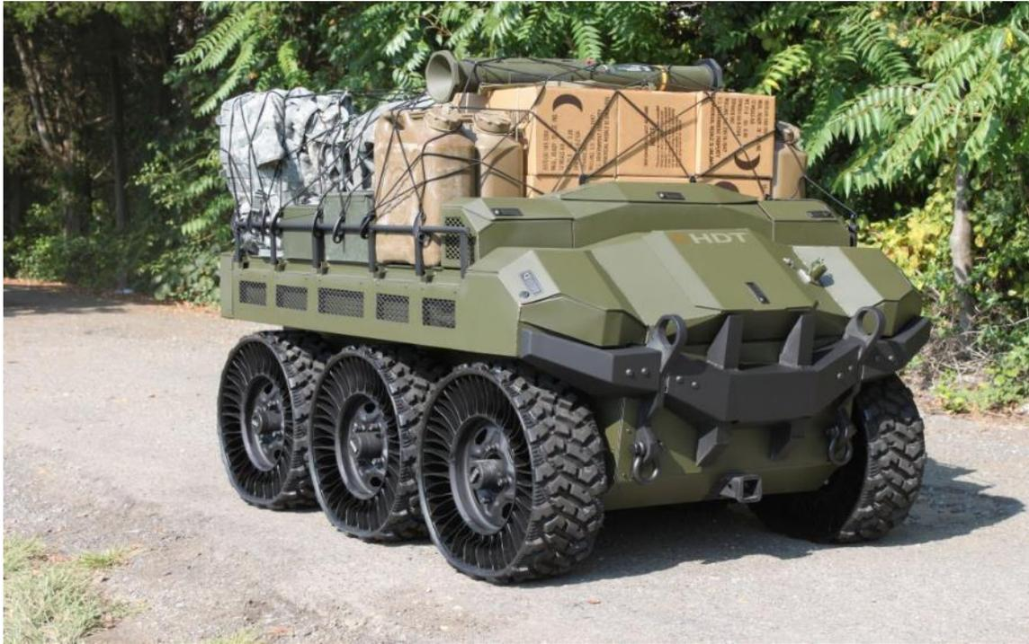
Seen here is a rugged 6x6 load-carrier (Mule) for dismounted infantry. Closely matching the mobility of infantry, the Hunter WOLF can traverse narrow trails, steep slopes, and dense jungles. Using only internal fuel, the vehicle has a 100 km (60 mile) range and 72-hour endurance. The vehicle's JP-8 / electric hybrid powertrain provides both a "silent drive" and "silent watch" capability. Included in this robot is a Polar 20 kW DC generator.
