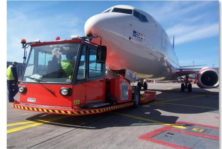
This Kalmar hybrid tow tractor incorporates a Polar Power 26 kW DC generator. Hybrid tow tractors can cost less to manufacture than conventional technology.
