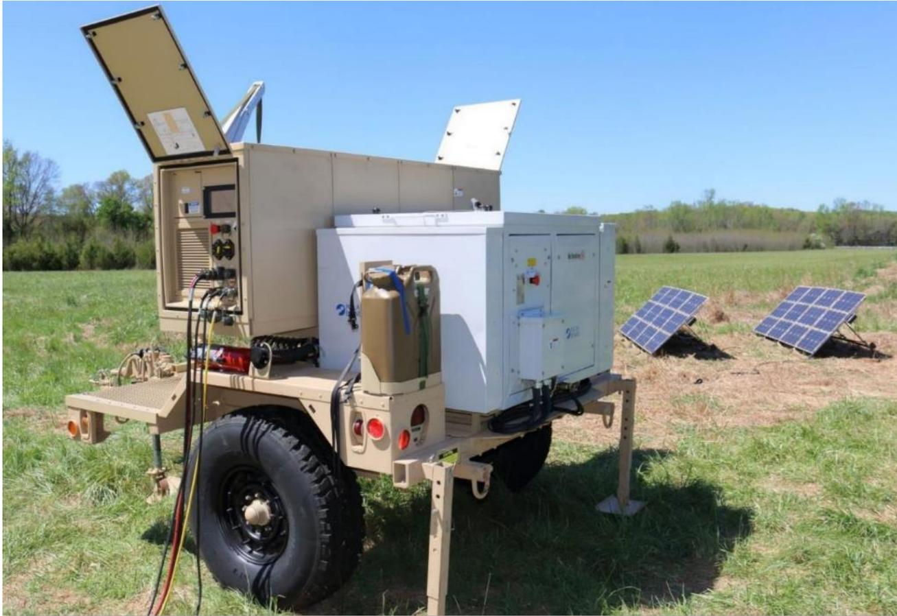
Small Unit Sustainment System, or SUSS, provides temporary power for shelters, communications, oil and mining work camps, and military expeditions.
