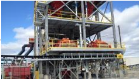
Wet Plant Cleans and Sorts Product
