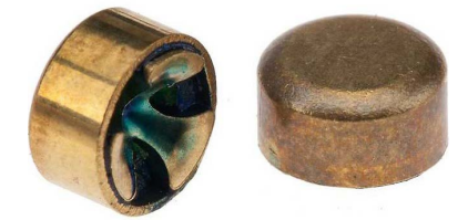
The lead-based primer compositions used widely in small caliber ammunition poses human and environmental hazards during manufacturing and use. MIC primer formulations and manufacturing approaches mitigate these risks, eliminating up to 12 tons of lead annually.
