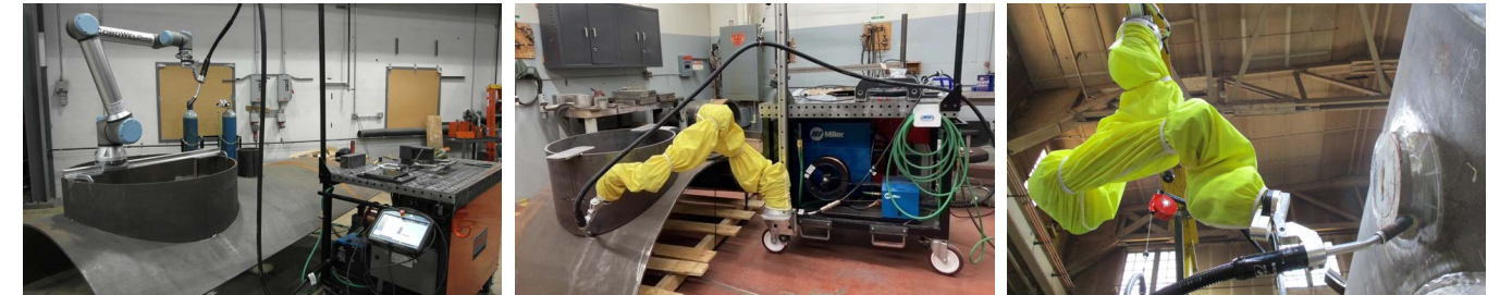
CTC's solution to address manufacturing challenges included modifying the existing track (left), cart (middle), and gantry (right) and installing a magnet to improve the Cobot's positioning and reach around the weldment.
