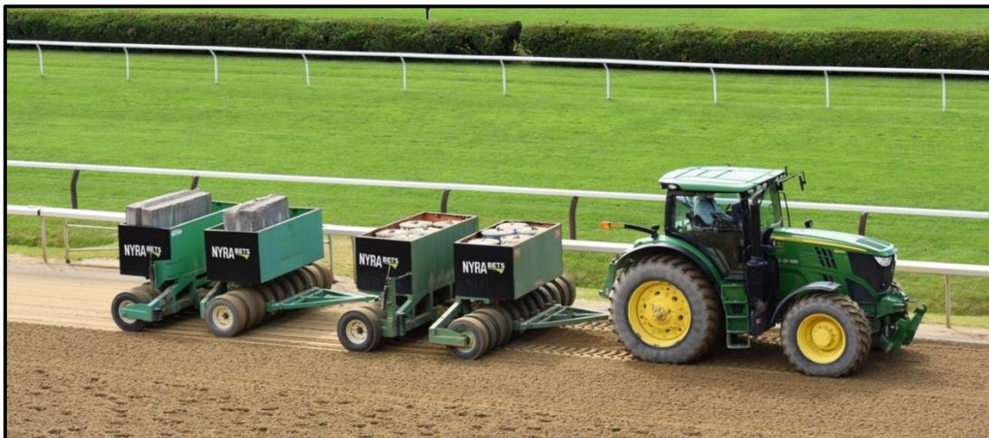
**Figure 3.** Rollers being pulled by a tractor over the Saratoga Main track to compact the freshly harrowed surface. (Photograph by Scott E. Palmer)
