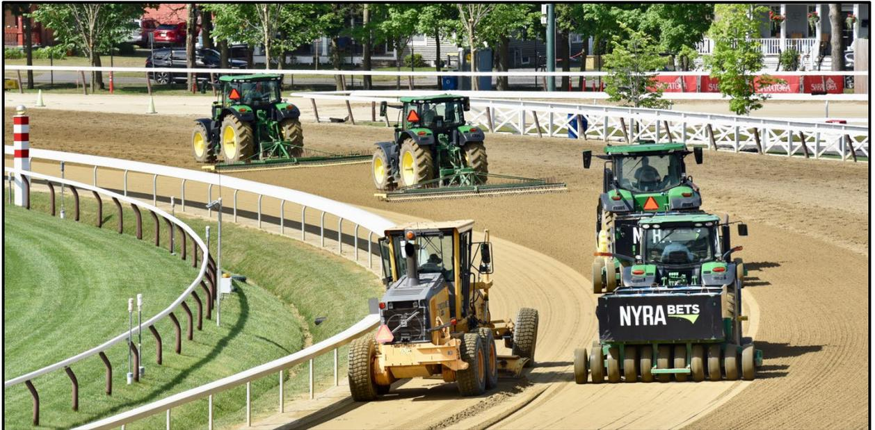
*Figure 9. State-of-the-art racetrack maintenance equipment is used daily at the Saratoga Race Course to condition the dirt racetracks for both training and racing. (Photograph by Scott E. Palmer)*
