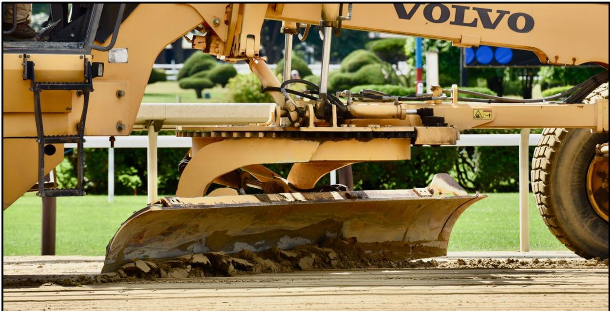
*Figure 1. A motor grader being used to shape the surface of the Saratoga Race Course to grade.
