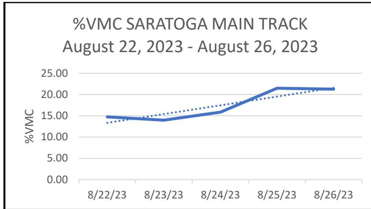
**Figure 18.** Percent Volume Moisture Content (%VMC) of the Main Track in the days leading up to Travers Day (August 26, 2023) during the 2023 Saratoga Race Meet. The dotted line is a positive trend line for increasing moisture content of the track in the days leading up to the feature races on August 26, 2023.
