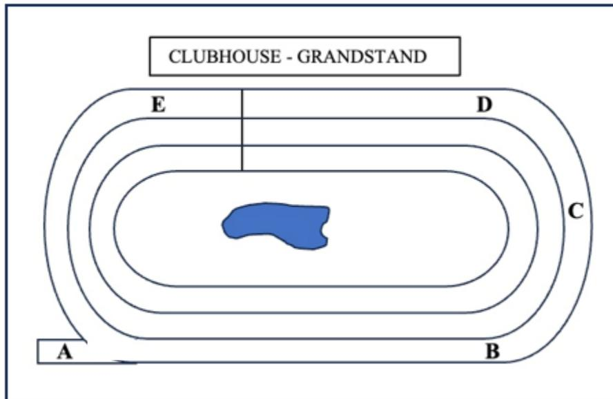
**Figure 19.** Percent VMC was measured at five locations around the Saratoga Main Track. Samples were obtained at (A) the 7/8-mile chute, (B) the 5/8-mile pole, (C) the 3/8-mile pole, (D) the 1/8-mile pole and (E) the 15/16-mile pole.
