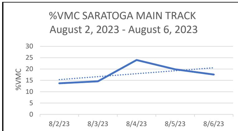
**Figure 17.** Percent volume moisture content (%VMC) of the Main Track in the days leading up to Whitney Day (August 6, 2023) during the 2023 Saratoga Meet. The dotted line is a positive trend line that represents accumulation of moisture in the racing surface leading up to the feature races on August 6, 2023.
