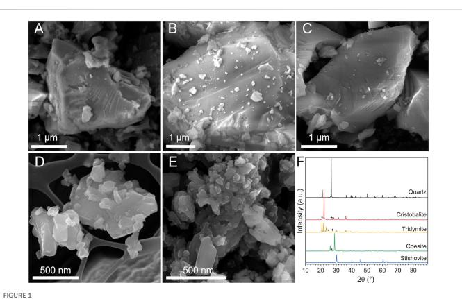
Morphology and crystallinity of the CS polymorphs. (A−E) Micrographs obtained by FESEM analysis: (A) quartz, (B) cristobalite, (C) tridymite, (D) coesite (background: grid of the stub), and (E) stishovite particles. (F) XRPD patterns of the CS polymorphs: ◆quartz and \*other contaminants.
