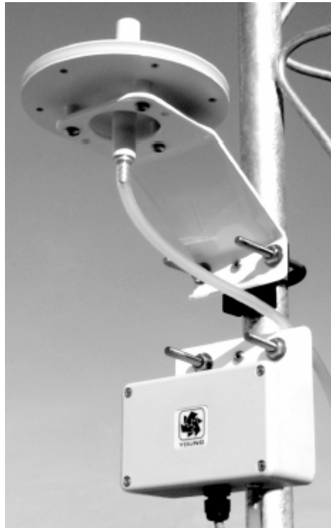
Figure 7.4 Tower-Mounted Barometer with Pressure Port. Source: http://www.youngusa.com
