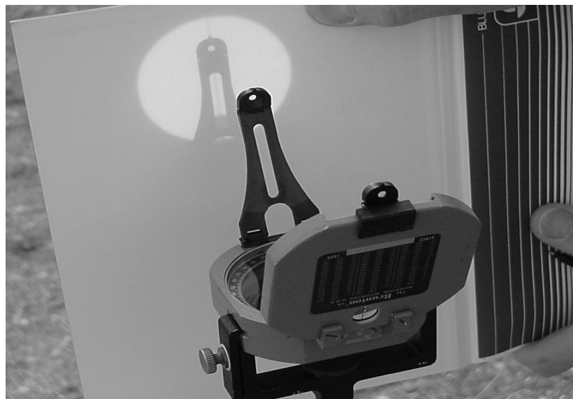
Figure 2.16 Projection of Sun's Reflection Using a Brunton Pocket Transit
