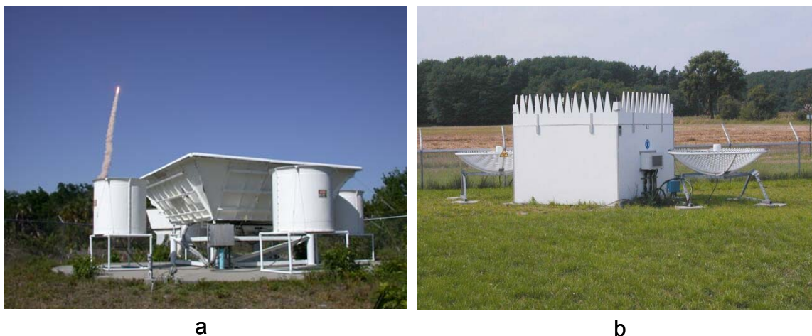
Figure 8.8 Photographs of (a) a Radar Wind Profiler with a RASS and (b) a Sodar with a RASS
