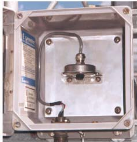
Figure 7.3 NEMA 4X Enclosure. Source: http://www.climatronics.com/pdf/products/sensors/102270.pdf
