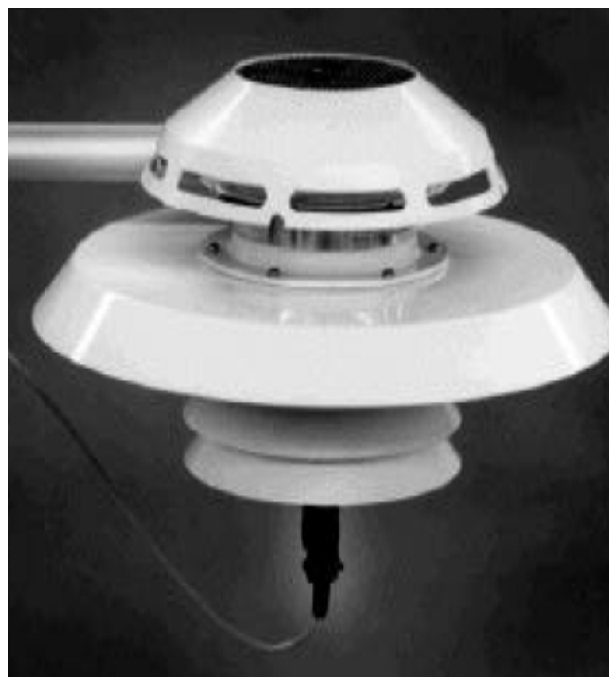
Figure 3.3 A Motor-Aspirated Shield. Source: < http://www.metone.com/ >
