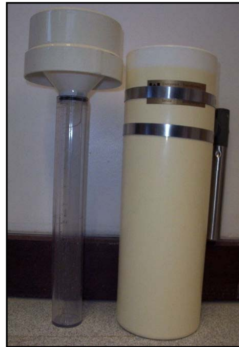
Figure 4.1 Cylinder Precipitation Gauge. Source: <22H http://www.rap.ucar.edu >
