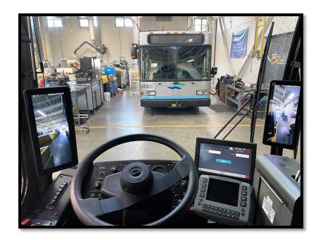
Monitors are mounted to optimize vision for driver / operators.
