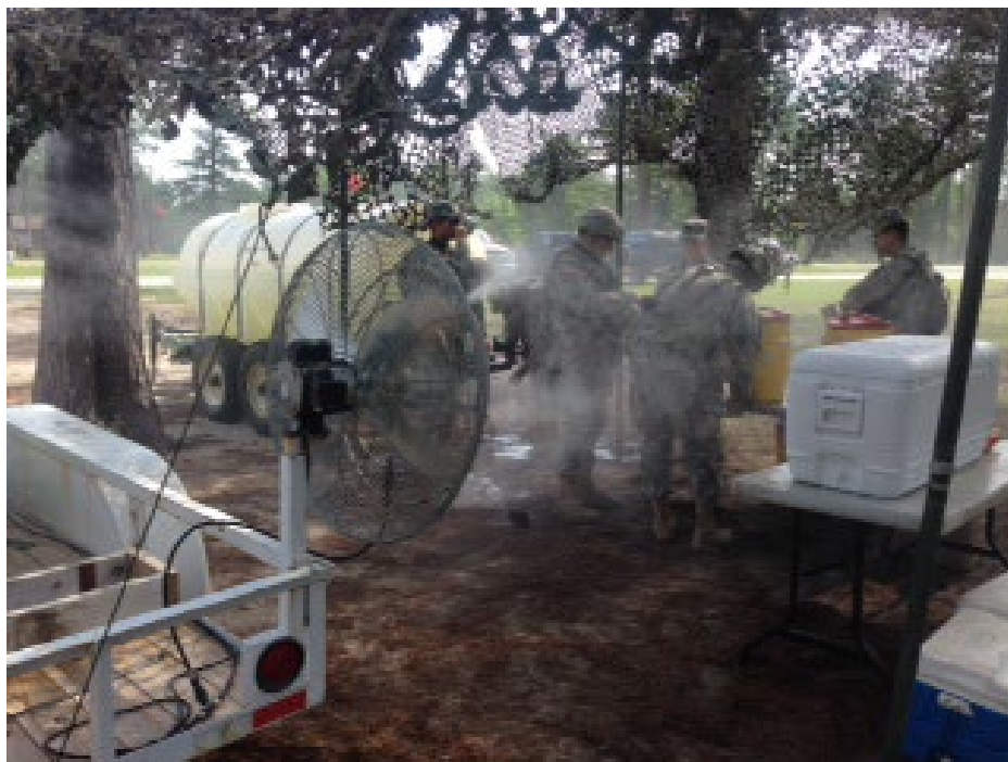
Figure E-4. Cool zone with misting fan, water resupply, and arm immersion cooling system
