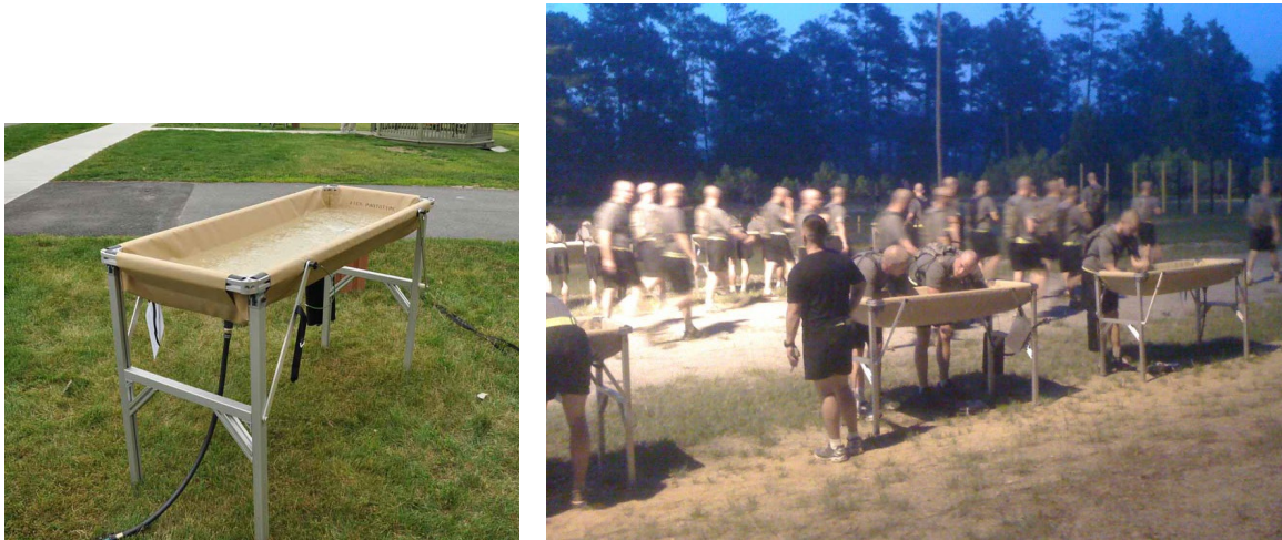
Figure E-1. Prototype arm immersion cooling system units
