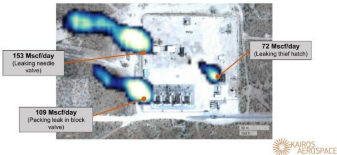
Figure 3: Three confirmed leaks observed at a compressor station facility in the Permian Basin.
