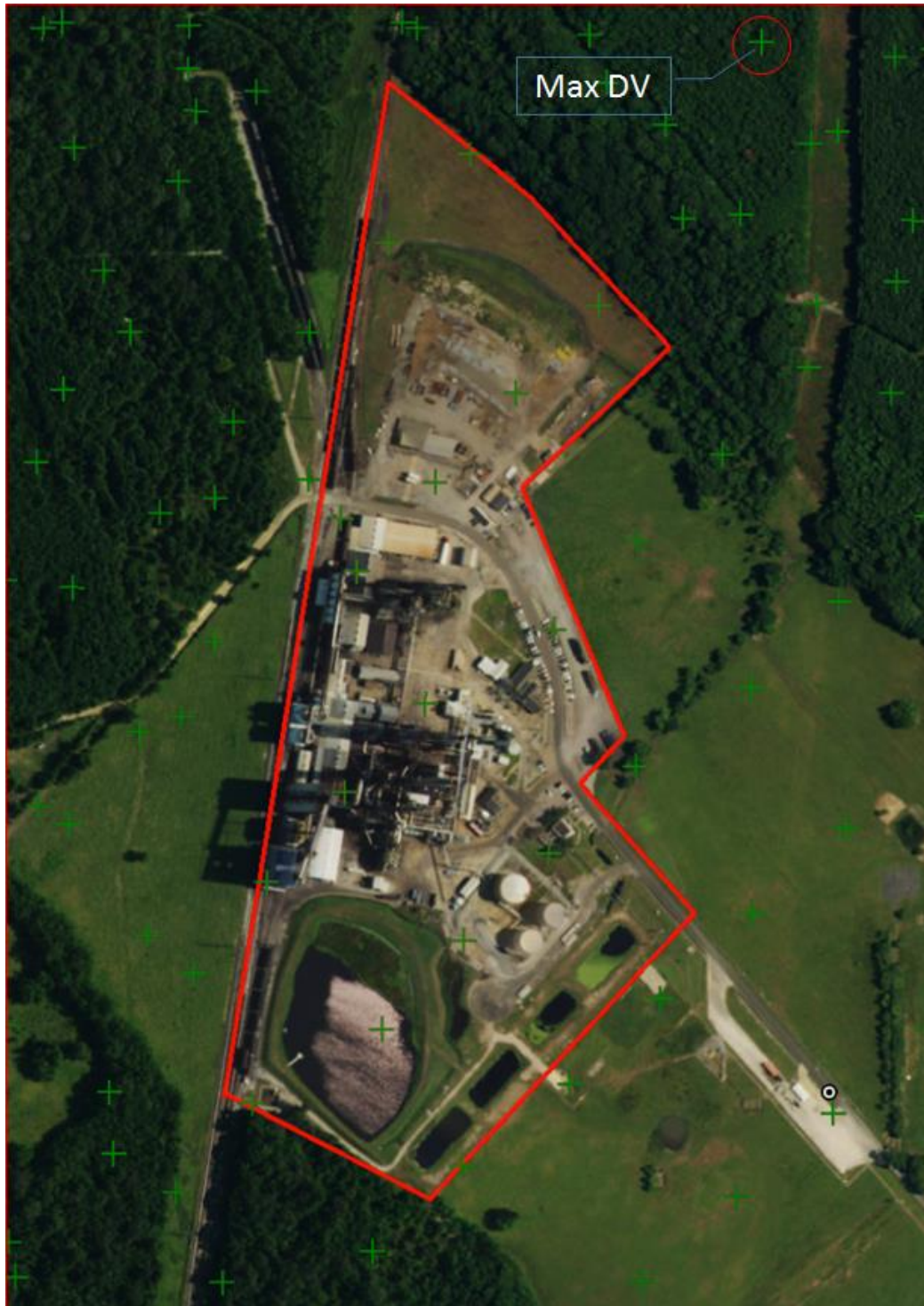
Figure 12: Near-field Receptor Grid for the Ville Platte Plant Area. The green “+” symbols represent the locations of receptors around the Cabot Ville Platte facility with the location of the maximum design value indicated by the red circle. Some receptors are evident within the facility fenceline itself (red boundary) and were included in the design value calculation using the modeled results.
