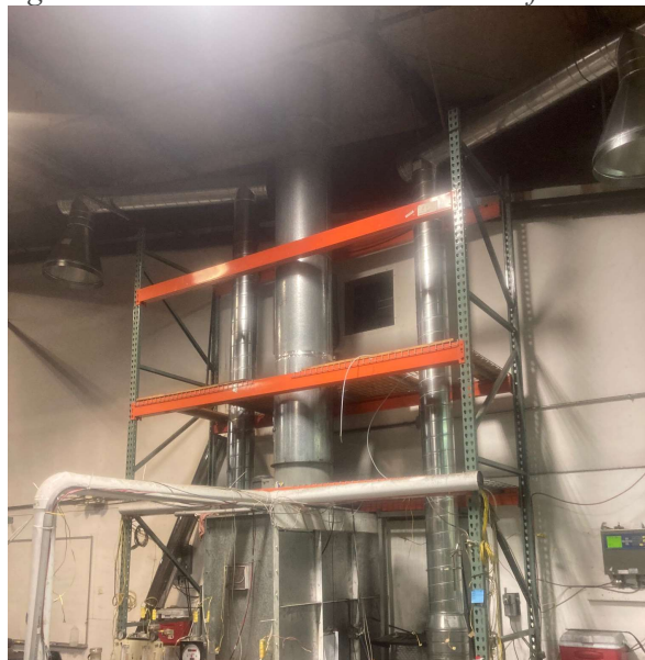
Figure 1. HLS 10" Dilution Tunnel used for mixing tests.
