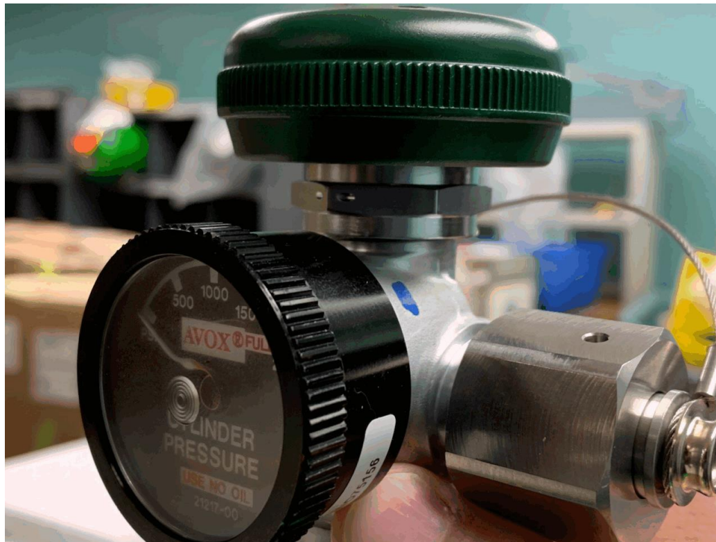
FIGURE 7 MARK ACCEPTABLE Cylinder & Valve Assembly (CVA) WITH A BLUE PAINT DOT
