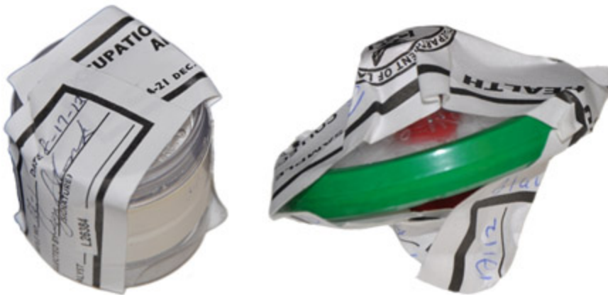
Figure E-4. Correctly sealed cassette with Form OSHA-21 covering inlet/outlet ports maintaining sample integrity.
