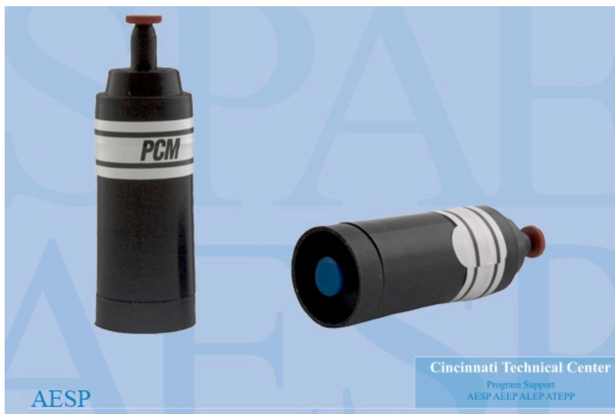
Figure 5. 0.8- \mu\text{m} pore size, 25-mm diameter MCEF cassette in an electrically conductive cassette assembly with 50-mm extension cowl. The end cap of the cassette visible on the right includes a blue Luer type plug. The entire end cap must be removed to allow open face sampling.
