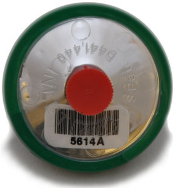
Figure B-4. Inlet View of a Filter Cassette (open to atmosphere, pointed downward during sampling)
