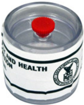
Figure E-3. Incorrectly sealed cassette allows access to inlet/outlet ports after sample has been taken.
