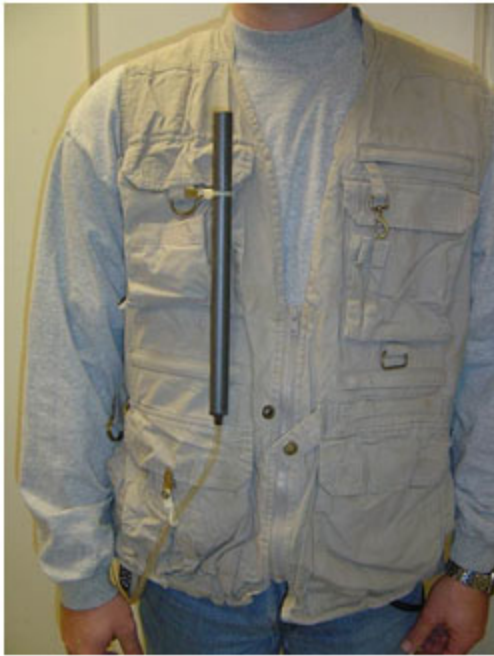
Figure 8. Large protective tube cover for sorbent tubes in series (photo courtesy of NIOSH)
