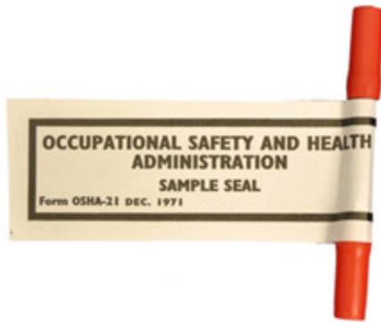
Figure E-2. Incorrectly sealed charcoal tube. End caps can be removed allowing sample integrity to be jeopardized without disturbing the seal.
