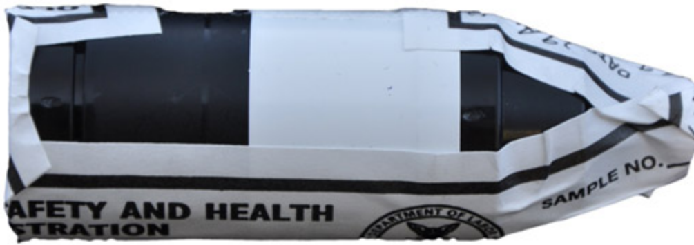
Figure E-5. Standard asbestos cassette (25mm) correctly sealed with a Form OSHA-21.
