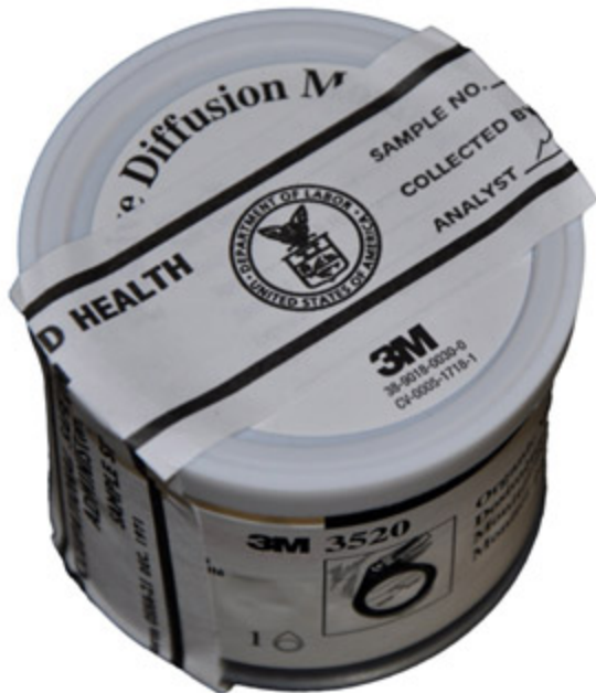
Figure E-7. Correctly sealed 3M passive monitor
