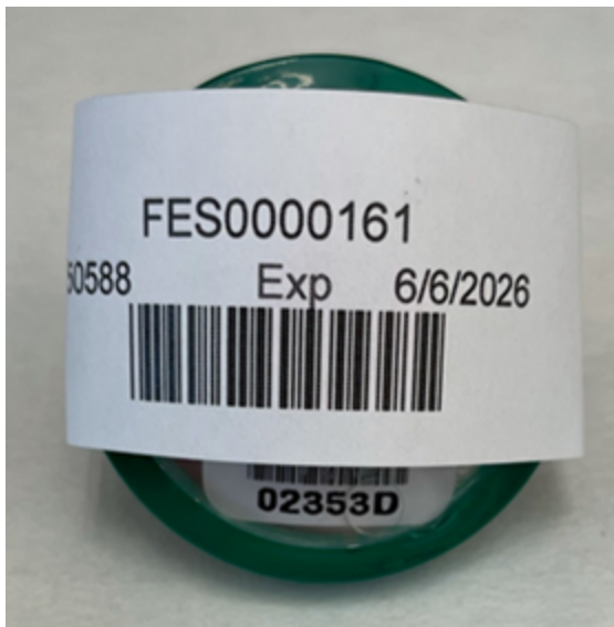
Figure B-5. Barcoded lot number and expiration date of filter cassette (discard prior to sampling)
