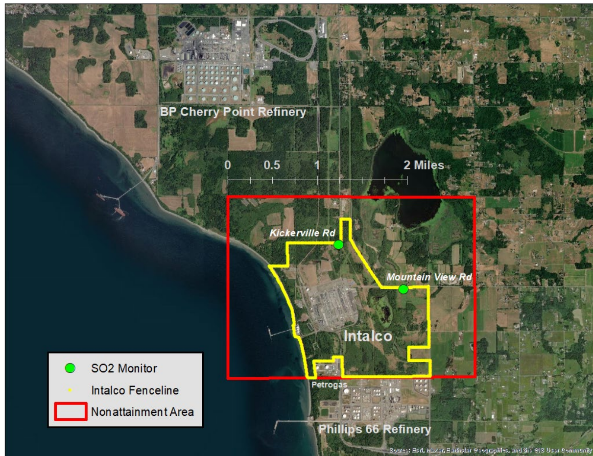
Figure 1. Intalco SO 2 nonattainment area boundary, SO 2 monitoring sites, and Intalco fence line
